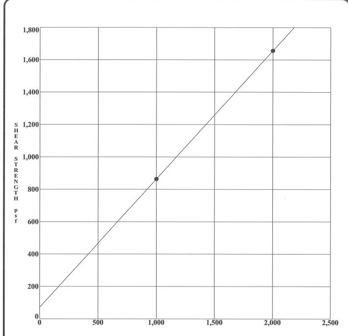
Cohesion Calc. (psf): 72 Friction Angle Calc. (°): 38 NORMAL PRESSURE, psf
