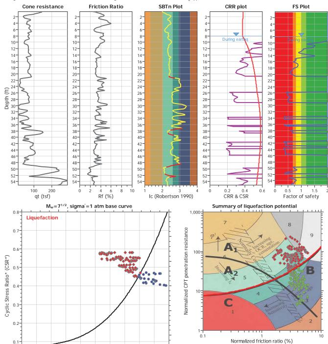
Zone A<sub>1</sub>: Cyclic liquefaction likely depending on size and duration of cyclic loading Zone A2: Cyclic liquefaction and strength loss likely depending on loading and ground
