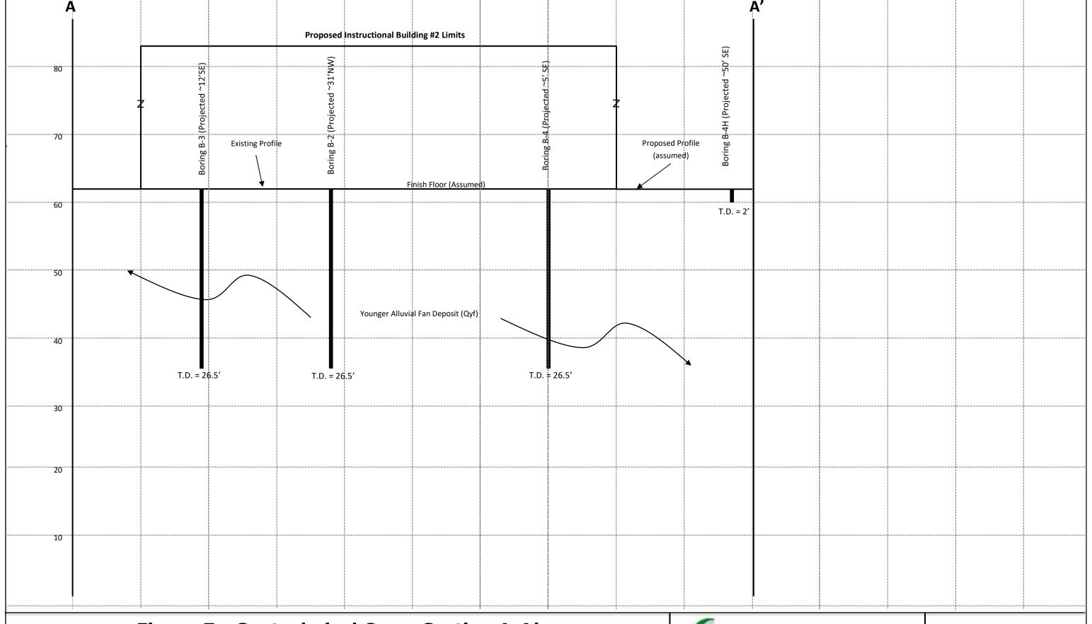
Figure 7 - Geotechnical Cross Section A-A'
