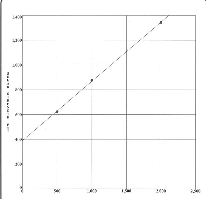
Cohesion Calc. (psf): 390 Friction Angle Calc. (°): 26 NORMAL PRESSURE, psf
