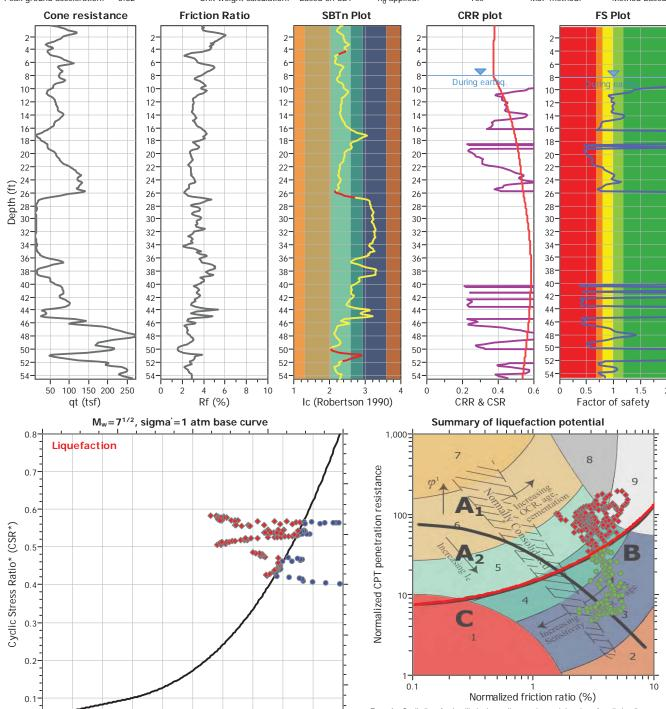
Zone  $A_1$ : Cyclic liquefaction likely depending on size and duration of cyclic loading Zone  $A_2$ : Cyclic liquefaction and strength loss likely depending on loading and ground geometry
