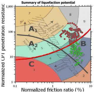
Zone A<sub>1</sub>: Cyclic liquefaction likely depending on size and duration of cyclic loading Zone A<sub>2</sub>: Cyclic liquefaction and strength loss likely depending on loading and ground geometry
