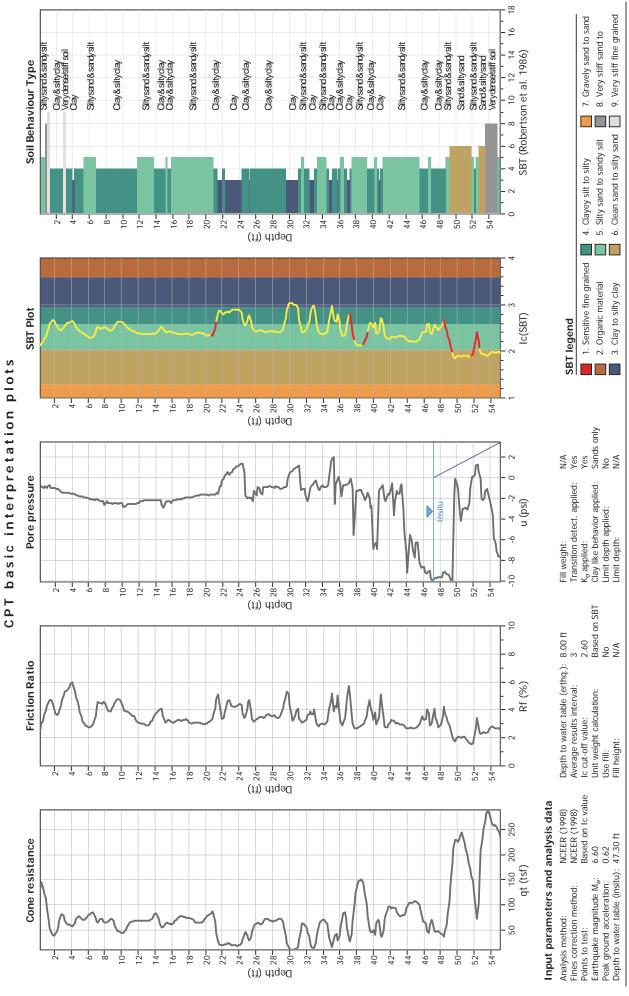
Project file: C:\Users\rshrestha\Box Sync\Geosphere-R Drive Folder\Geotech Projects by Number\3600-3699\91-03615-A Compton CCD\Liquefaction Analysis\Liquefaction- (GWT 8 ft with transition and weighted Volu Strain).clg CLiq v.1.7.6.49 - CPT Liquefaction Assessment Software - Report created on: 12/15/2015, 2:10:23 PM
